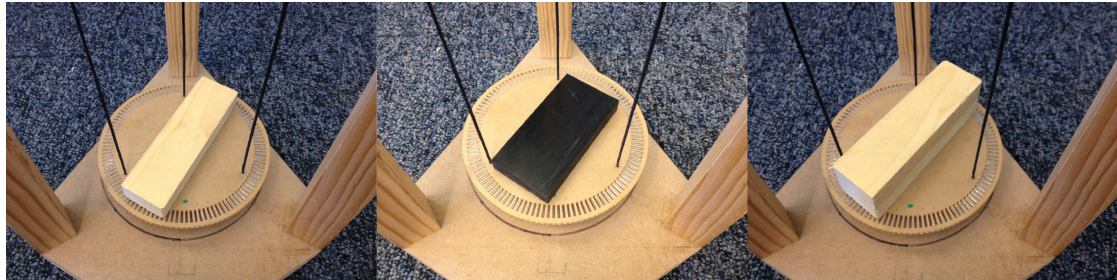
Figure 7.3: Block samples. From left to right: single block, ABS block, and two wooden blocks.
